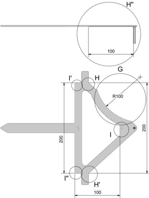
102.3. - Gauge 2, Front Impact Thickness Zone AA' to BB' (not used on integrated padding)
